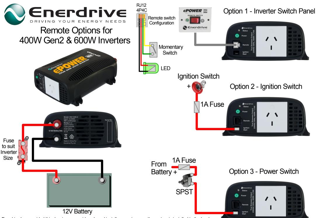
Enerdrive has provided this drawing as a guide only and installers must ensure the system is installed to the local requirements for fuse protection and wire sizing. If you have any questions please call; Enerdrive on 07 3390 6900
